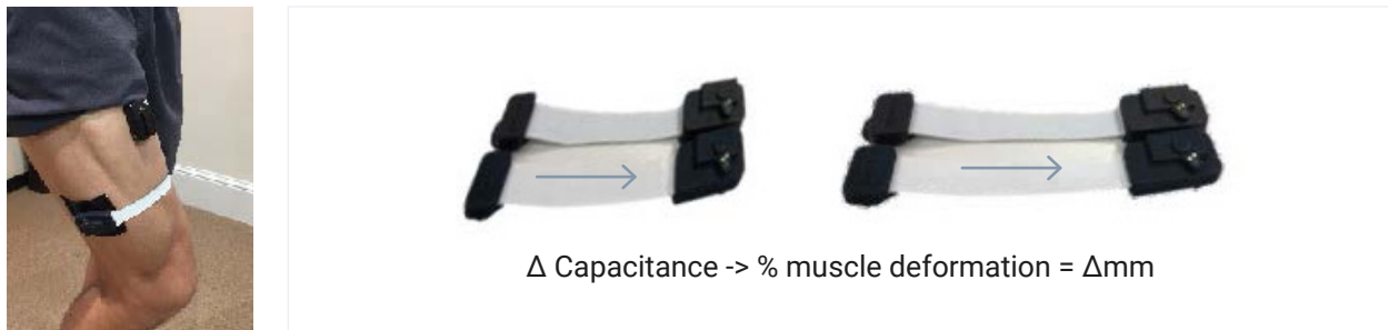
Figure 2. Illustration of the FIGUR8 sMMG sensor application for muscle output.
